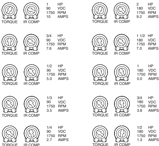
Figure 19. Recommended TORQUE and IR COMP Settings
