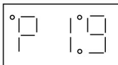
Once the desired parameter number is found, press the **Mode** button to display the present parameter setting. The upper right-hand decimal point will begin blinking, indicating that the present parameter setting is being displayed, and that it can be changed by using the ▲ and ▼ buttons.
