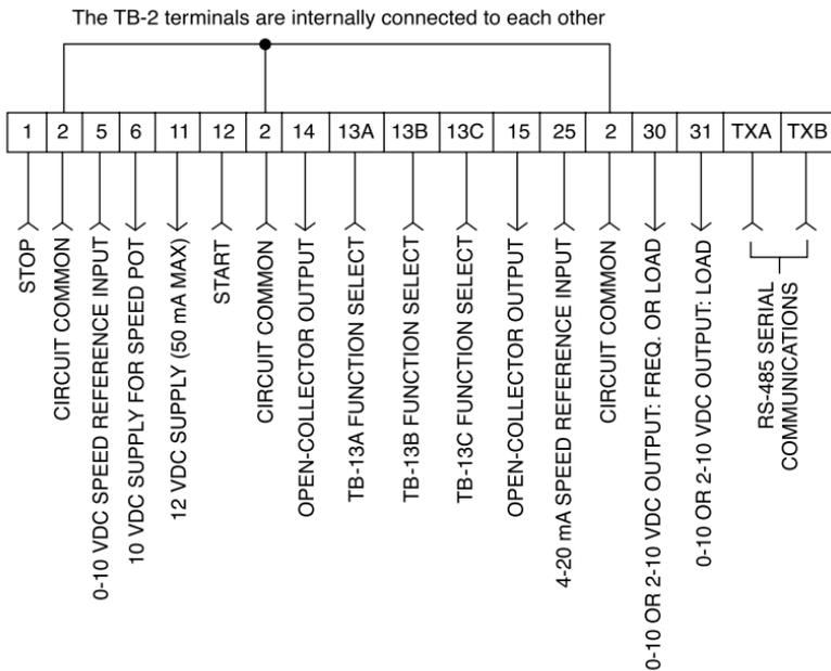
**NOTE:** The function of terminals TB-13A, TB-13B, TB-13C, TB-14, TB-15, TB-30, and TB-31 are dependent on the programming of certain parameters. Refer to Section 15.0 - DESCRIPTION OF PARAMETERS.
